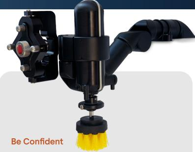
The Reach Alpha Probe and Brush is a dualfunction manipulator built to conduct remote inspection and maintenance activities in harsh, subsea environments. Capable of cleaning away sediment and organic build-up on a surface, as well as collecting accurate data determining corrosion levels, the Alpha Probe and Brush unit is reducing risk and cost factors associated with inspection requirements in Oil and Gas industries.
